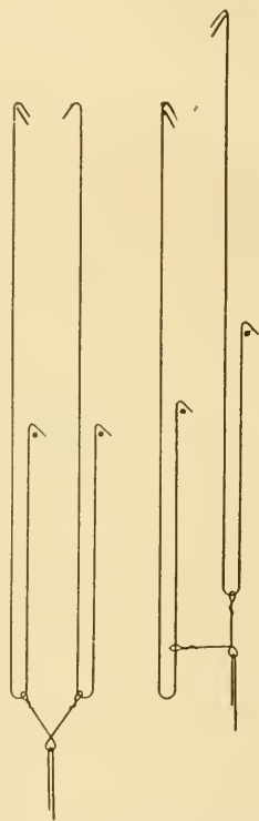
Fig. 26. Showing Connection of Neck Cords to Hooks.
